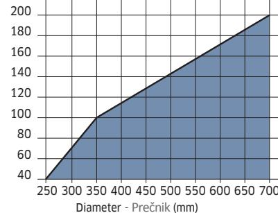
Maximum depth of cut based on the blade diameter.
