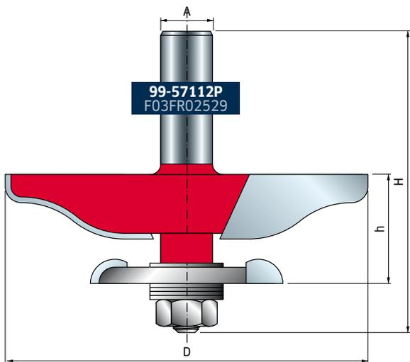
To produce the inner raised panel router the panel on all four sides but ensure that **the two across vein sides are routed first**.
