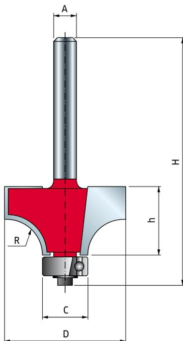
By simply ordering the **Ball bearing 3102M AA9P** (Ø 3/8") and the **Step washer FX07M AA9P** you will be able to obtain a different profile.
