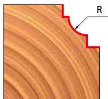
With bearing  $\varnothing$  9,5 mm
