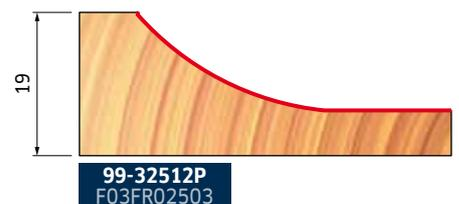
To produce the inner raised panel router the panel on all four sides but ensure that **the two across vein sides are routed first.**
